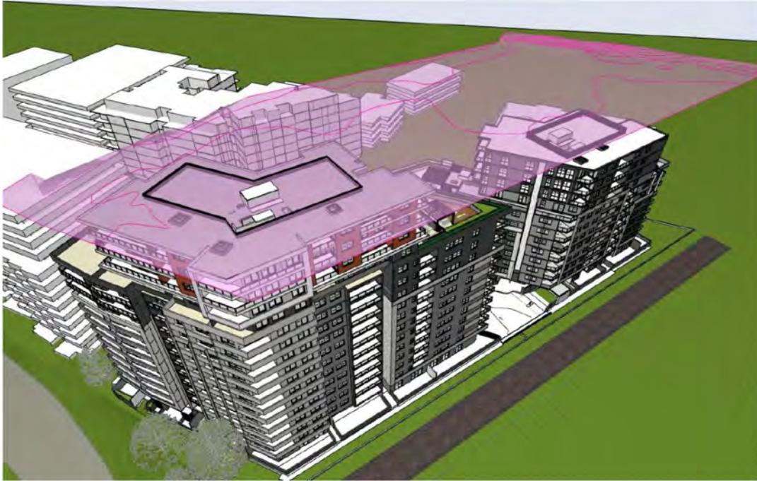
Figure 2: Height plane at 50m from existing ground level (Source: Zhinar Architects)
